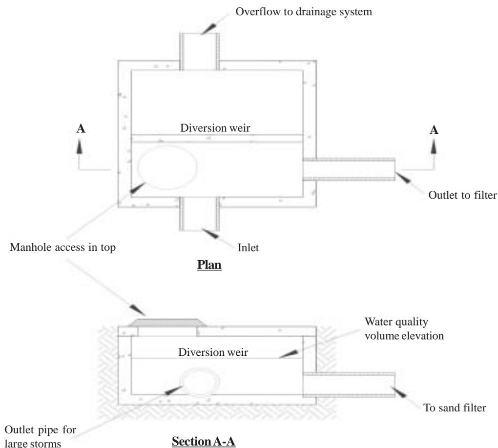
Figure 7-1 provides a typical detail of a flow diverter which can be used primarily for concentrated flow into a sand filter. Rain gardens should have an overflow spillway set above the water quality storm or an overland flow path for larger events.
