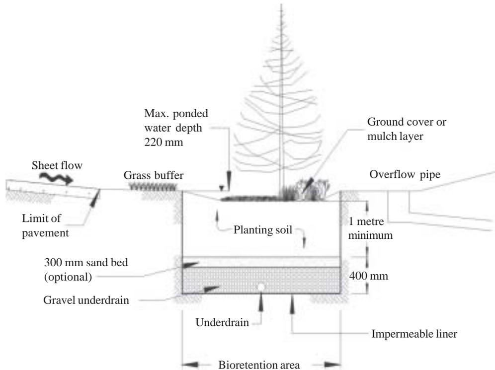
The gravel underdrain will collect and distribute treated excess runoff. A properly designed underdrain system helps keep the soil from becoming saturated. The underdrain system consists of a gravel layer with a 100 - 150 mm perforated piping system. There should be a minimum of 50 mm of gravel cover over the perforated pipe.
