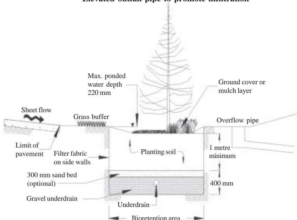
underdrain system. It is not recommended that a filter cloth be placed between the planting soil, sand bed and gravel underdrain because the fabric represents an area of potential clogging. A small amount of soil migration may be expected but the system will stabilise. Filter fabric (open weave in stable soils; impervious in unstable soils) should be used, at least on the side walls, to prevent migration of adjacent soil particles into the rain garden.
